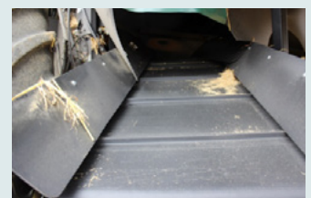
Figure 2: One of the two chaff deck conveyors
