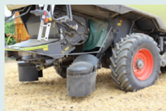
Figure 1: Installed chaff deck
